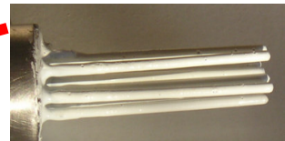
Signal was significant even though coating appeared intact after 14-day exposure
