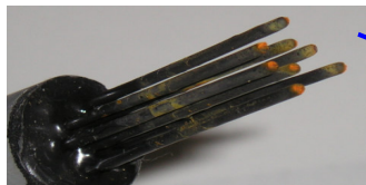
Rust observed on all defected areas after 7-day exposure
