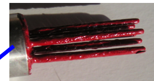
A small area of coating peeled off after 7-day exposure
