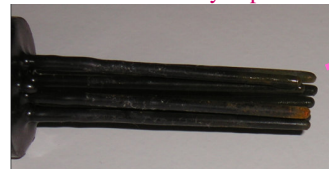
Rust observed on defected areas after 7-day exposure
