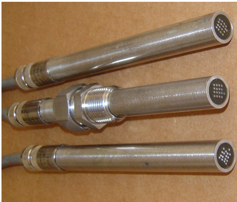
Figure 2. Typical coupled multielectrode array sensor probes.
